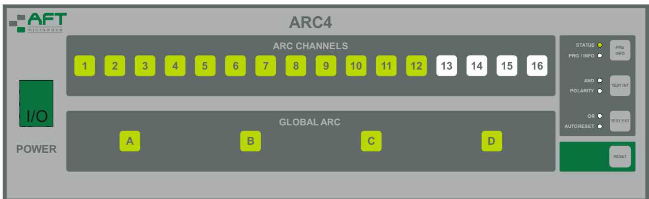
Fig. 6.2: Front panel status display example 1: normal operation, no active alarms, slots 13 to 16 empty
