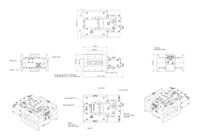
Fig. 1: Interface dimensions, all dimensions in mm.
