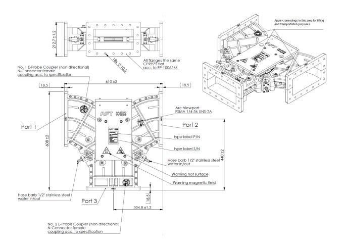
Fig. 1: Interface dimensions, all dimensions in mm.
